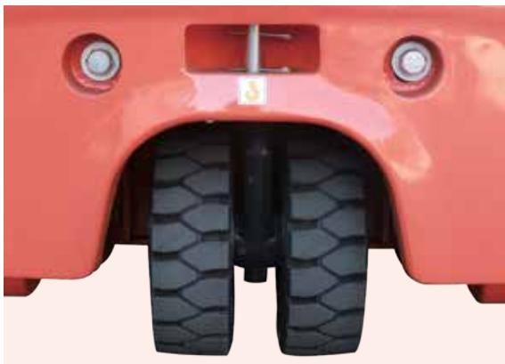
The rear wheels have been upgraded from the original 15X4 1/2-8 to 140/55-9 tires to increase their carrying capacity.
