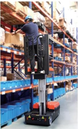
Both models are equipped with automatic closing doors preventing the operation of the truck when doors are opened. High-strength aluminum alloy profiles help to achieve great stability due to the lowered gravity center.
