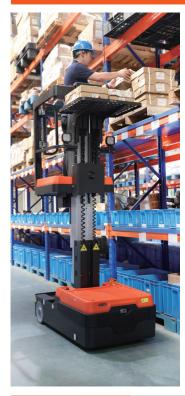
While platform is raising to its maximum height, the maximum available lift and drive speeds will go through three steps of speed settings according to the following lift height ranges for the platform: 0-500mm, 500-1500mm, 1500-3318mm to ensure the truck's stability and operator's safety.
