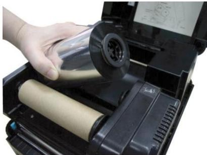
5. Insert the left side first. Please be noted that the bigger hub side with 4 ribs must be installed toward the right side of ribbon mechanism.
