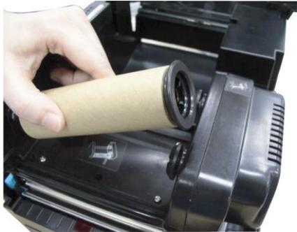
4. Install a ribbon on the ribbon supply spindle. Mount the ribbon supply spindle on the rear hubs.
