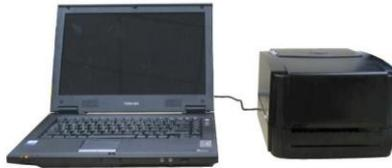
4. Plug the power cord into the power jacket at the rear of the printer, and then plug the power cord into a properly grounded receptacle.
