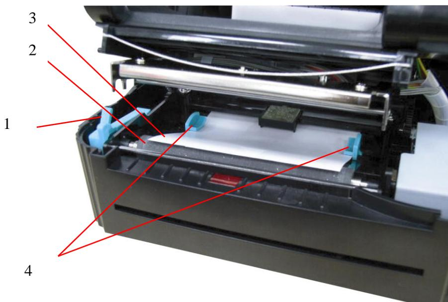
1. Printer Carriage Release Lever
