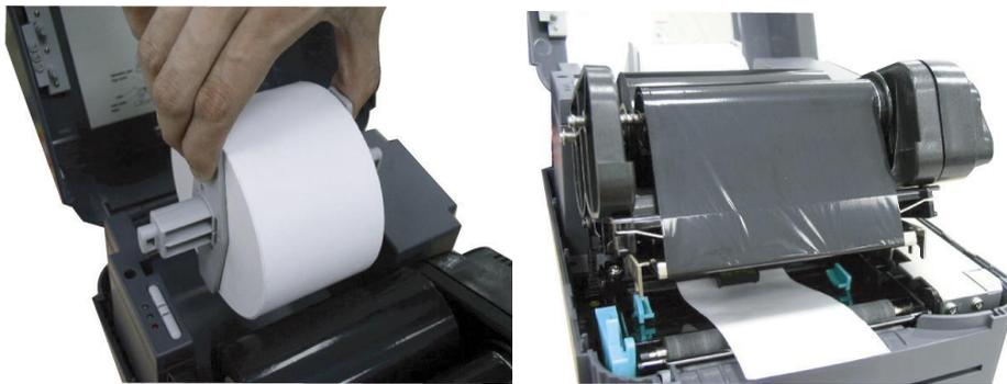
5. Adjust the label guide to fit the width of the media.
